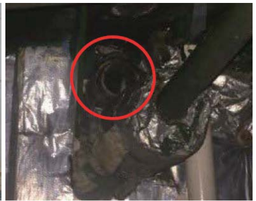
Hole in A-60 class Bulk head
